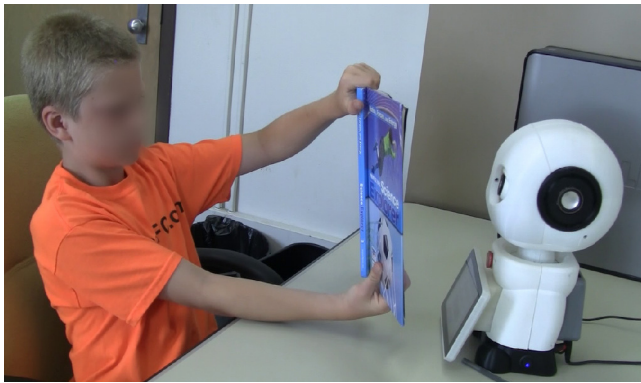
Figure 3: Child scanning an AprilTag by pointing the textbook towards the robot's camera (red circle on robot torso).
